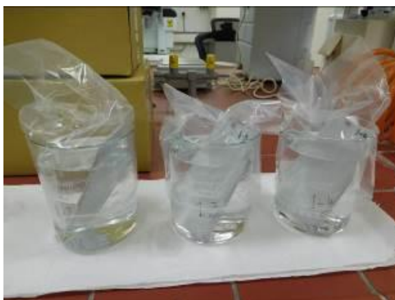
Figure 10: Test coupons in immersion
