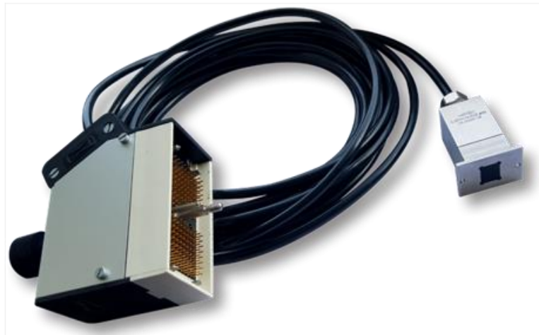
Figure 2: A typical phased array ultrasound transducer for data acquisition in ultrasound NDE inspections and experiments. A phased array transducer consists of many small piezoelectric acoustically active elements that are independently excited both in the process of firing ultrasound beams and in the process of collecting the ultrasound waves reflected within the tester materials and configurations.
