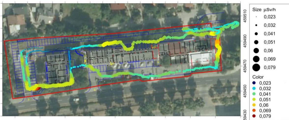
Figure 3: Heatmap generated with early version of FRAS system around IMROH building. (Note: Measured values are not representation of total ambient dose equivalent as detector employs proprietary natural background rejection – NBR system.)
