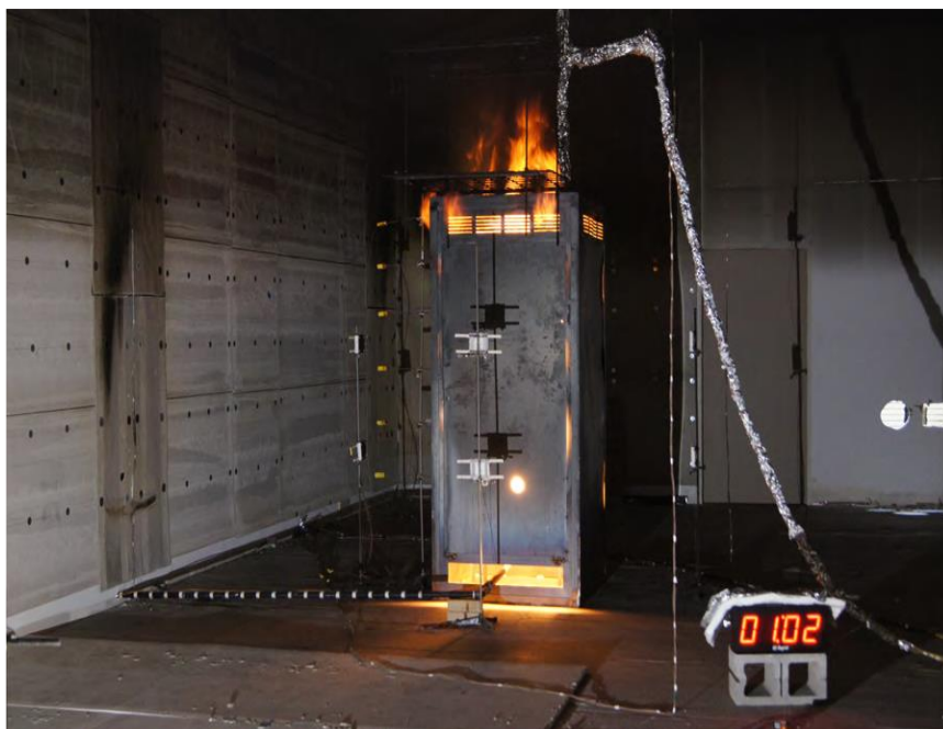
Figure 3: Electrical cubicle fire testing experiment
