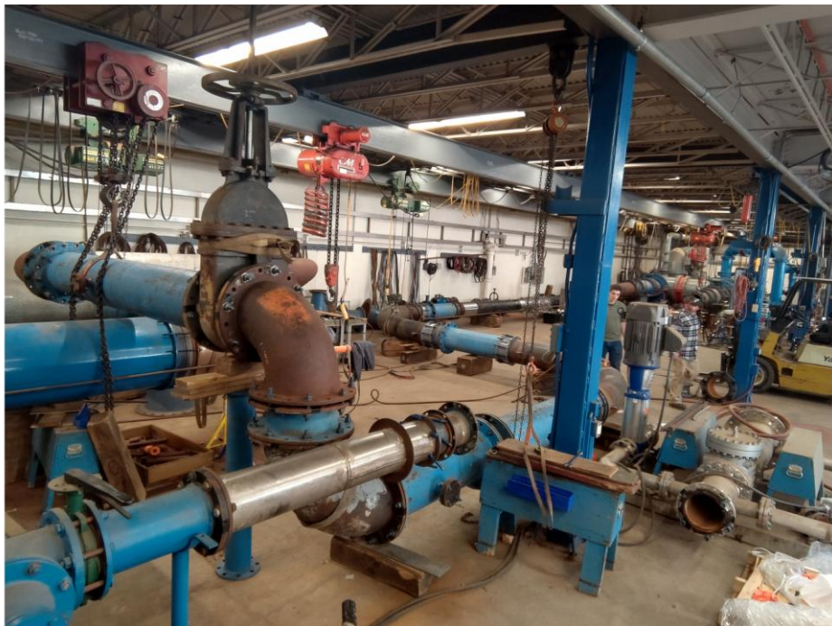
Figure 5: 1:1 model of NEK FW system assembled at Alden Research Laboratory
