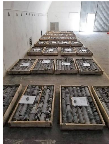
Figure 6: Drilling and core samples from borehole 198 m deep [3]
