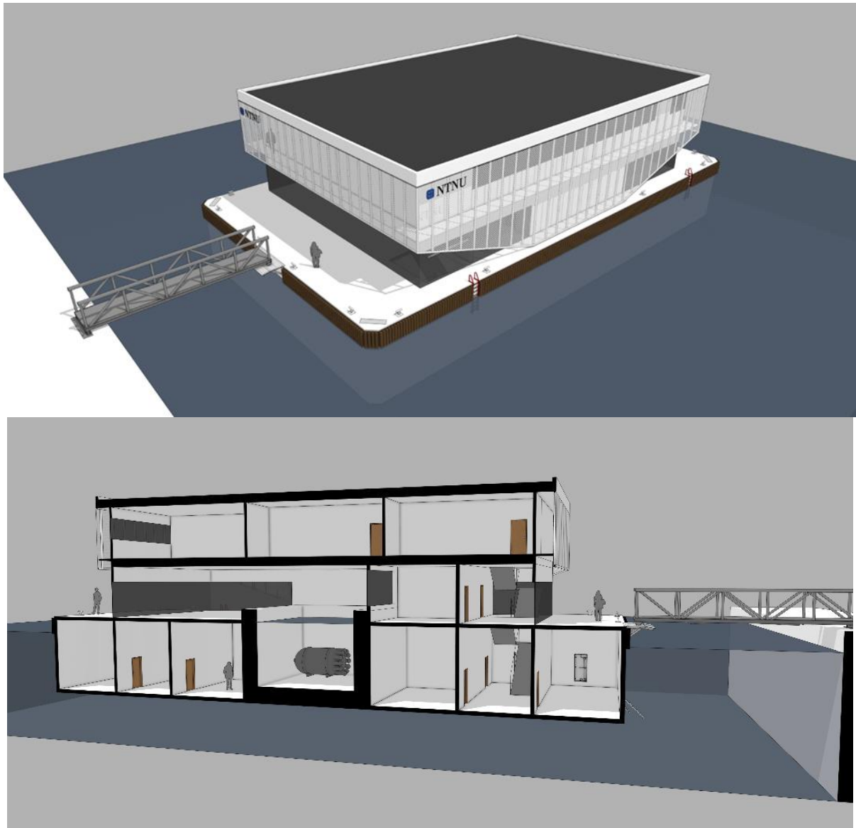
Figure 7: Alongshore FNPP developed for test reactor at Norwegian University of Science and Technology in Norway and cooperation with Ulstein Betongindustri AS.
