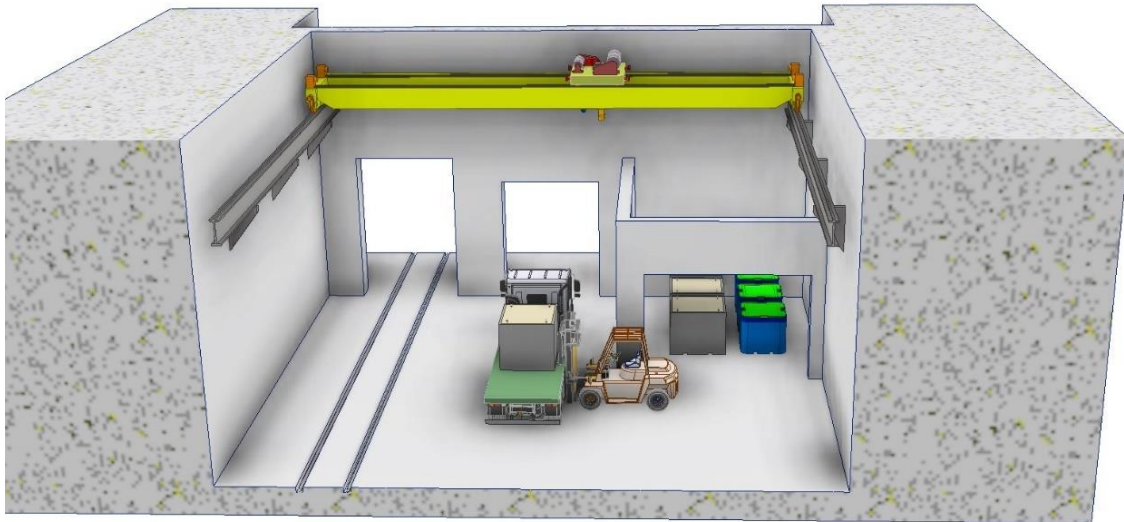
Figure 4: Handling of WP with RAW in the reception and reloading hall using a forklift – loading onto a truck for transporting RAW to the disposal horizon
