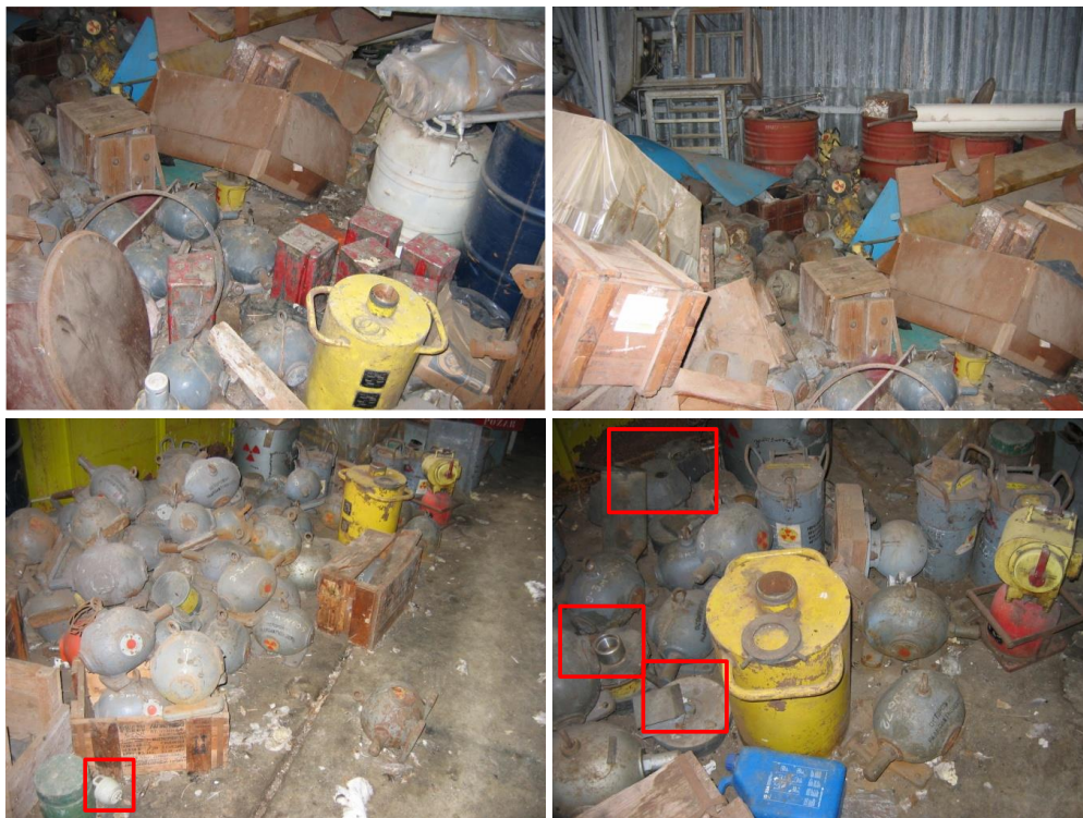
Figure 5: Photos of the interior of hangar H1- used sealed industrial radioactive sources
