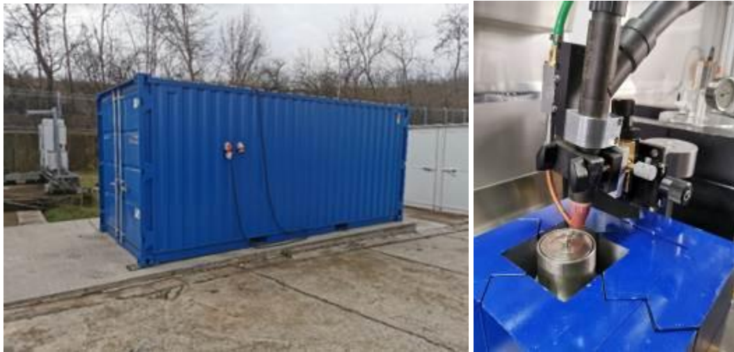
Figure 22: Mobile unit for welding collection capsules, automatic capsule welding machine
