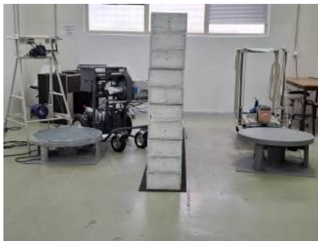
Figure 14: Equipment for non-destructive characterisation of RW with rotating stands
