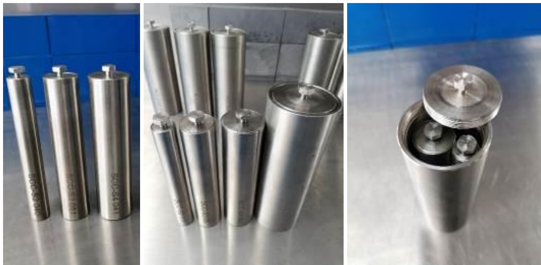
Figure 20: Stainless-steel capsules for conditioned sources showing the packaging of SCC-S2/S3/S4 capsules into an IAEA SCC-R L2 capsule
