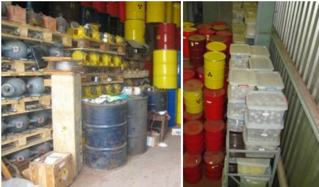
Figure 10: Industrial sources (DSRS) and SD stored in hangar H2
