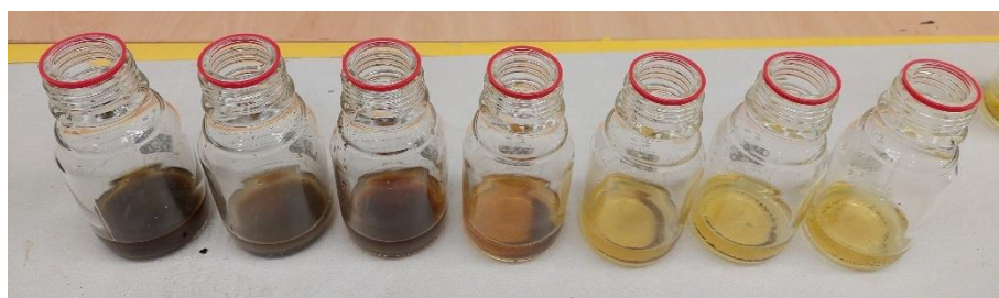
Figure 2: IEX destruction over time (left: initial IEX, right: destroyed IEX)
