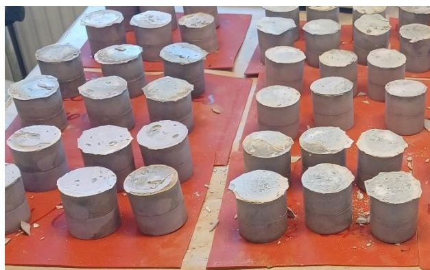
Figure 3: Photograph of the prepared cement samples made with concentrated liquefied IEX
