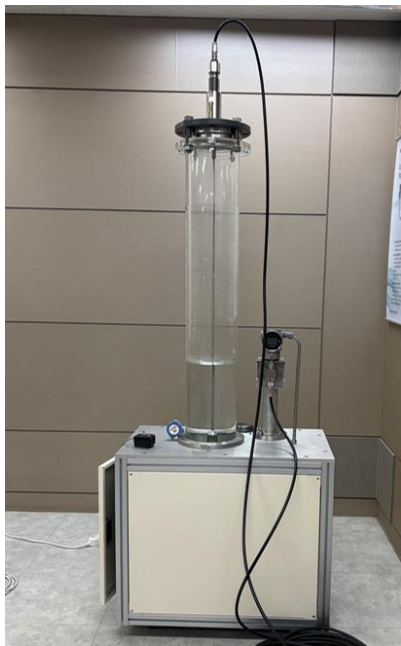
Figure 6: GWR 8m high water tank test and EMI test report
