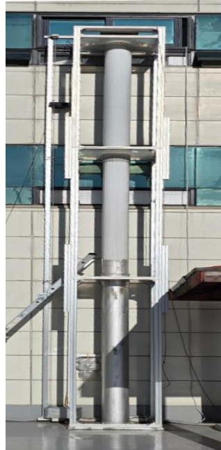
Figure 6: GWR 8m high water tank test and EMI test report
